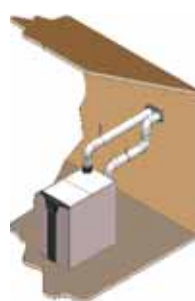
Direct Vent Sidewall
